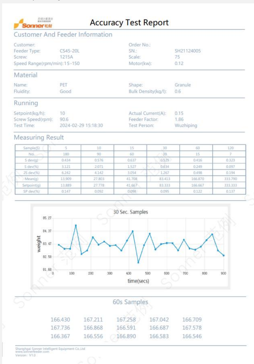
CFE45-1215A Typical Accuracy Testing Table
